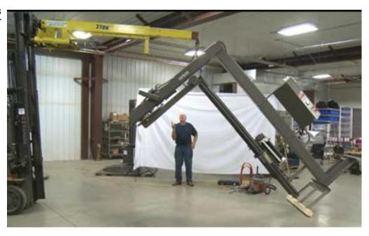
**3.** Your spotter can position the machine precisely while the lift is holding the tower vertically.
