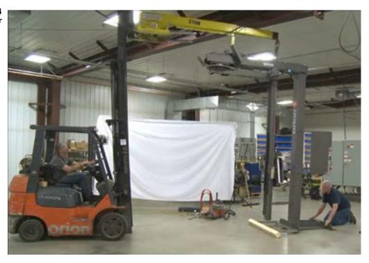
**4.** Remove the shipping feet while the machine is still held by the lift.
