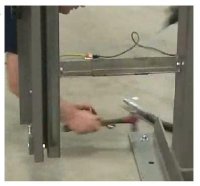
7. Once the machine is properly bolted down, loosen the tension to the crossmember.
