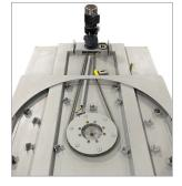
Robust Ring Bearing Support 6,000 lb. maximum load capacity,
