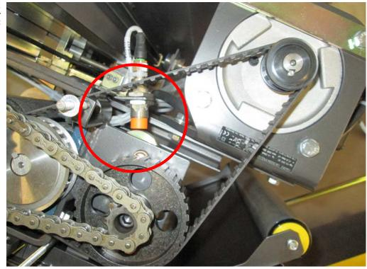
Figure 5 - 2 Proximity Sensor Adjustment
