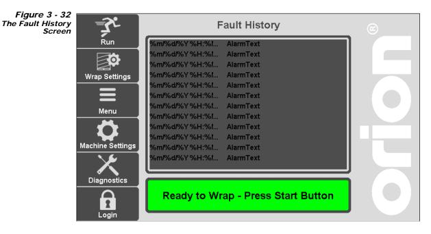
This is the Fault History screen. The screen displays the faults and the time they occurred.
