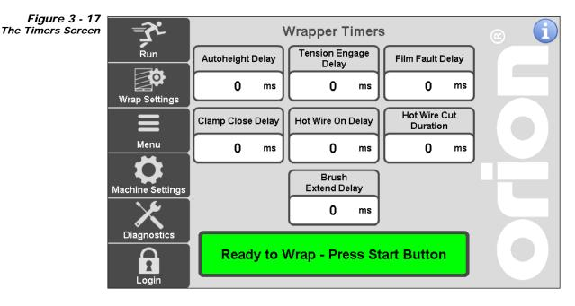
This is the Timers Screen. This screen allows adjustment of the timers involved in the machine cycle. See the Table below for descriptions and parameters of each setting.
