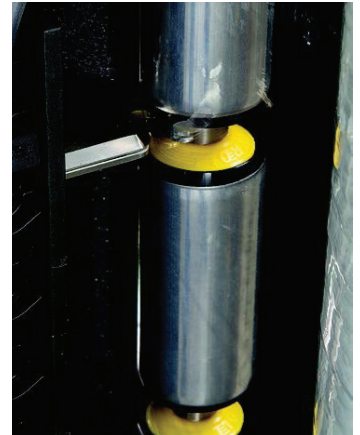
Figure 1 - A knife inserted on the carriage splits the film in two to strips of film which is then passed through the rollers system (See figure 2) to create the film bands.
