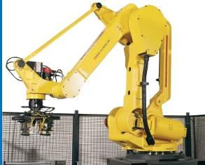
The robot is an electric servo-driven, four-axis model by FANUC Robotics. With an integrated mechanical and control unit, the M-410i (RJ3) series of robots provide high speed, high payload capability without sacrificing accuracy and repeatability. Capable of handling payloads up to 880 pounds (400kg) and axis speeds up to 300 degrees per second, the M-410i is the best-in-class solution for your automated palletizing / depalletizing needs.
