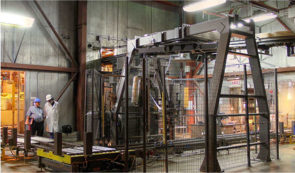
The Orion MA-X with custom conveyor helped Schwan's streamline frozen pizza handling and reduce labor costs.
