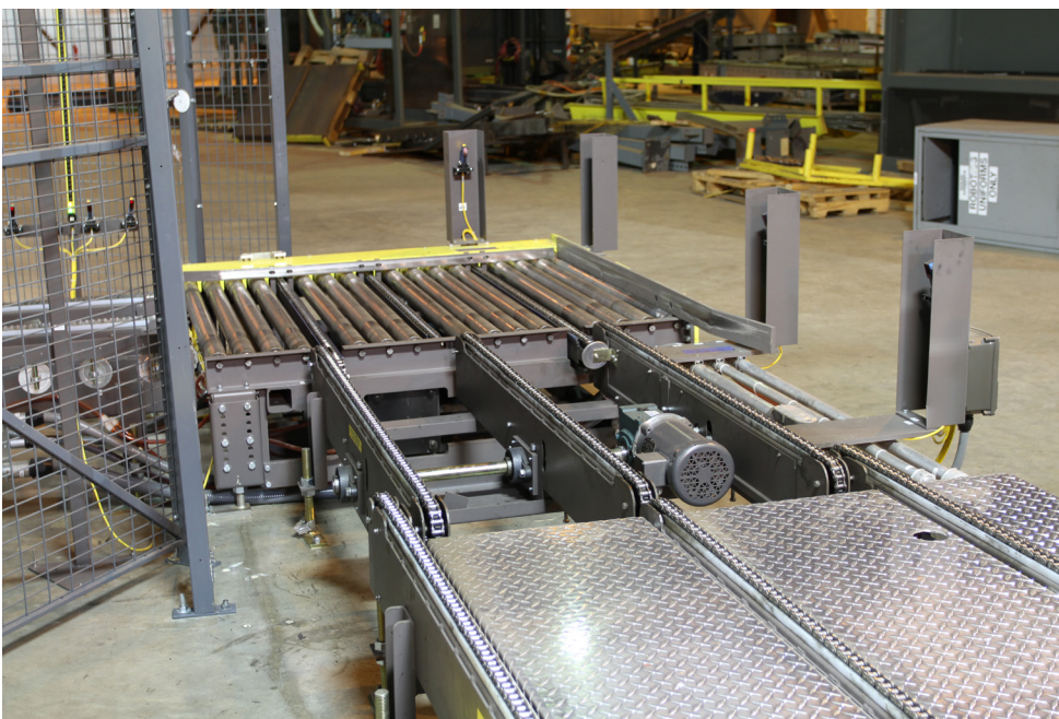
The chain transfer section of the conveyor is built with the highest quality components for heavy-duty operation and long term reliability.
