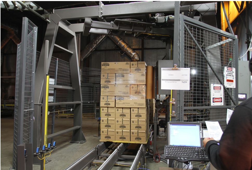
The Orion MA-X applies the stabilizing wrap on the pallet load, then secures the film tail with a wipe down brush. An operator will apply a label when the load is transported by.
