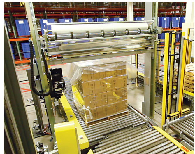
Once stretch wrapped, a top sheet is applied and the load reverses back to the turntable for another layer of protective stretch wrap.
