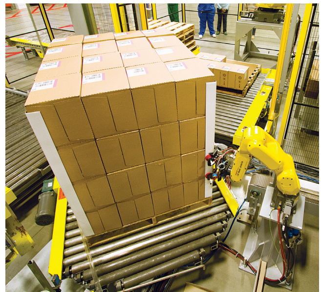
Prior to stretch wrapping, a single robotic arm picks up a cornerboard, applies adhesive and precisely places one on each of the four corners of the load.
