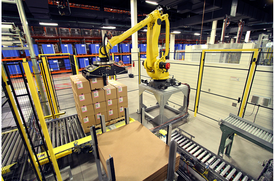
A Fanuc robot picks cases from the infeed conveyor to build pallet loads. A specially designed end of arm tool flips each case 90 degrees for proper orientation during shipment. The robot is also capable of staging empty pallets and placing slip sheets.
