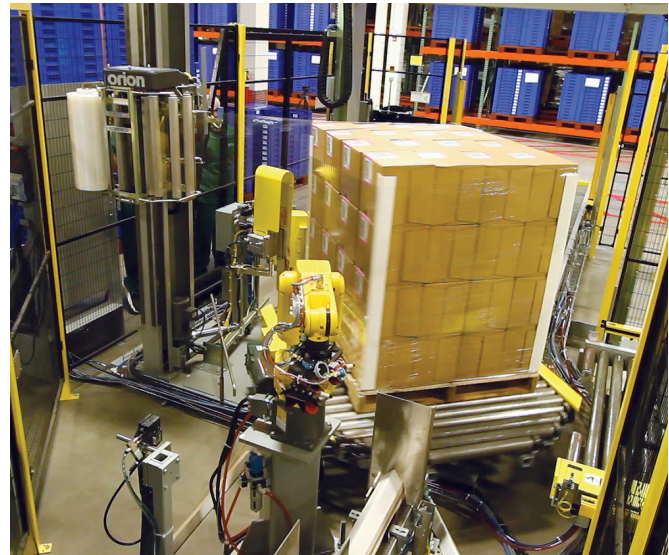
After the four cornerboards are applied to the pallet load, an Orion FA automatic stretch wrapper applies a tight, even wrap of film that has been pre-stretched 260%.
